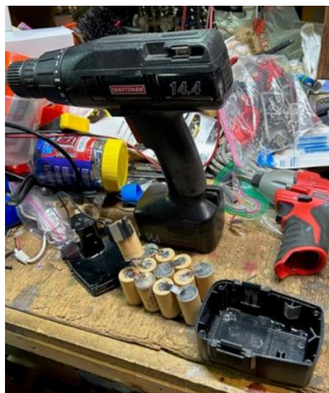
Upon opening up the Craftsman battery pack, I found really old NiCd batteries with corrosion.
