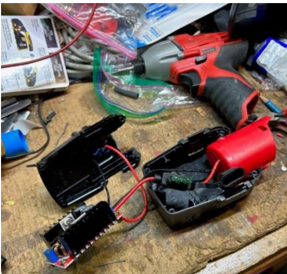
The BOOST converter can be seen.
