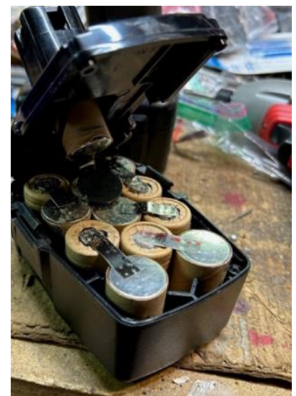
Upon opening up the Craftsman battery pack, I found really old NiCd batteries with corrosion.
