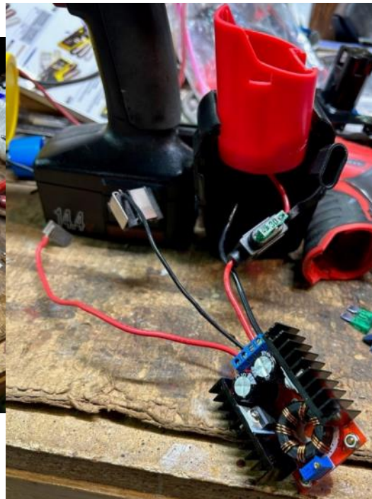
The BOOST converter can be seen.
